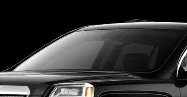
ACOUSTIC LAMINATED GLASS The windshield is engineered with acoustic laminated glass to help keep road noise from entering the cabin.
