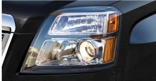
PROJECTOR-BEAM HEADLAMPS Terrain provides bright, focused illumination for confident visibility with integral projector-beam headlamps. For daytime illumination, Terrain offers LED daytime running lamps for excellent visibility and durability.
